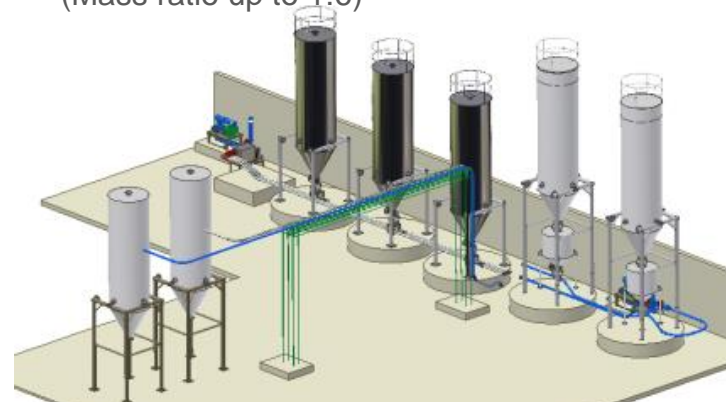
Bangkok PVC Co., Ltd. PVC door raw material conveying system PVC compound powder, Calcium carbonate powder
