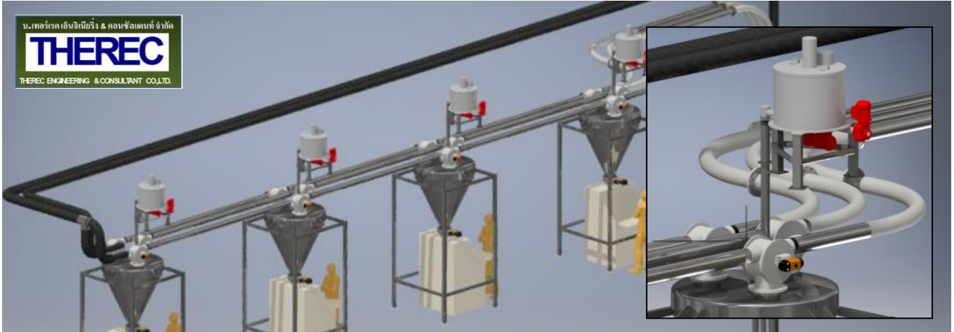
Saha Aree Industry Co., Ltd./ PVC and Calcium carbonate powder weighting system by Scale (Fill vent) valve
