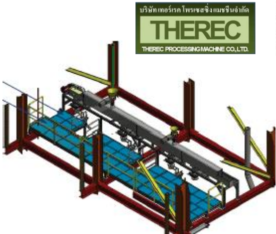
Quality Coffee Co., Ltd. / Nest Café Roasted coffee bean Bulk truck loading system With chain conveyor and loading bellow ,no need to move the truck during the loading period of time.
