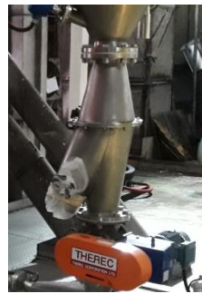
Air lock Rotary & Diverter Valve / Product Sampling Valve / Mitr Pukeaw Factory Sugar dust from vibrating screener. blow to packing machine
