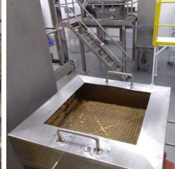
Lump Breakers / Mitr Puieng. / Brown Sugar
