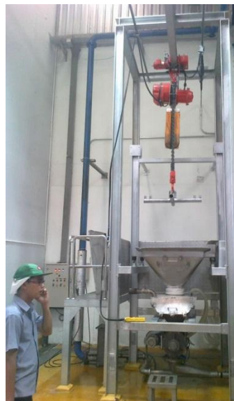
Big Bag Unloading station / Sugar TIPCO Food Co., Ltd.
