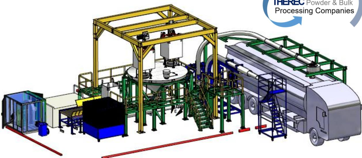
Full Bulk material handling system for powder and bulk processing line / Storage / Loading / Unloading / Weighing / Mixing / Sizes classifying
