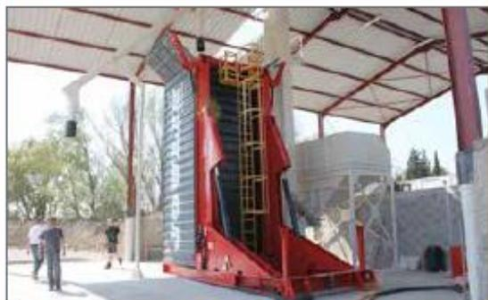
Kraft Foods in France uses an A-Ward container loader to load coffee beans into shipping containers for domestic storage.
