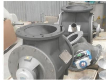
Non cutting Rotary valve (Granular Valve)
