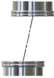
Off Set equipment IG = CL - 20mm (Minimum)
