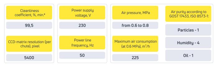
\* With the initial content of foreign materials of 2% or less and the volume weight of the product of 0.750 t/m<sup>3</sup>
