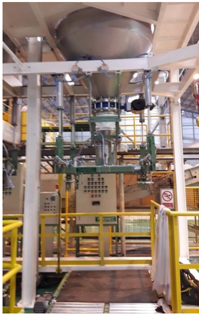
Bulk bag Filing Machine, High speed & Low speed type Available for all requirement
